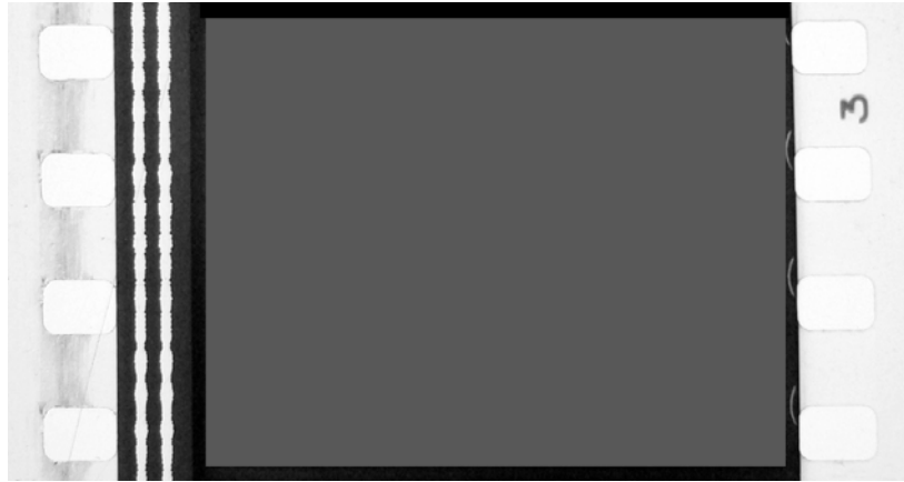
Figure 2.1: 35mm analog soundtrack (double bilateral variable area tracks)
